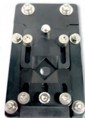
Figure 1: Micro sample holder for samples of 10 - 14 mm internal diameter or rectangular shaped samples; maximum diameter of the light beam for transmittance measurement is 5 mm
