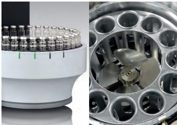
Figure 3: Air circulation incubator oven and sample tray of the HS-20
