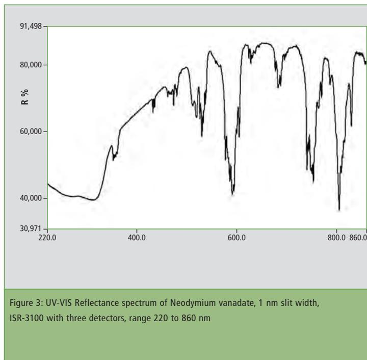
Figure 3: UV-VIS Reflectance spectrum of Neodymium vanadate, 1 nm slit width, ISR-3100 with three detectors, range 220 to 860 nm
