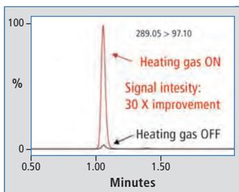
Figure 3: Effect of heating gas – MRM chromatogram of testosterone
