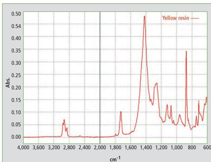
Figure 1: ATR spectrum from PVC resin measured with a diamond reflection unit
