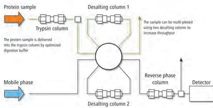
Figure 3: Flow schematics of the Perfinity iDP system
