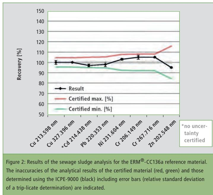
Figure 2: Results of the sewage sludge analysis for the ERM<sup>®</sup>-CC136a reference material. The inaccuracies of the analytical results of the certified material (red, green) and those determined using the ICPE-9000 (black) including error bars (relative standard deviation of a triplicate determination) are indicated.
