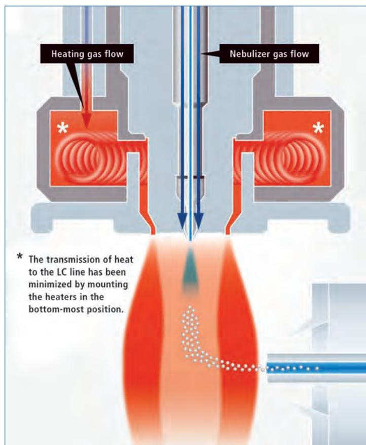
Figure 2: Illustration of the newly developed heated ESI source
