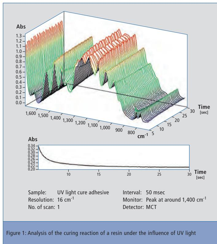
Figure 1: Analysis of the curing reaction of a resin under the influence of UV light
