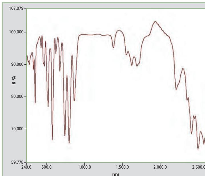
Figure 5: UV-VIS NIR spectrum from Neodymium phosphate  $\text{NdPO}_4$ , 5 nm measurement in the range from 240 to 2,600 nm
